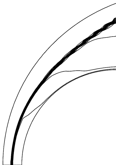
Fig. 8b Mach number contours (second-order accuracy in space).
