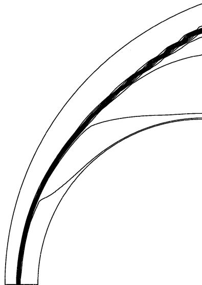
Fig. 8a Mach number contours (first-order accuracy in space).
